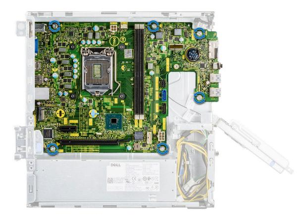
4 Connect the following cables to the system board- PSU cable [1], power switch cable [2], HDD SATA cable and HDD/ODD power cable [3], ODD SATA cable and PSU cable [4].
