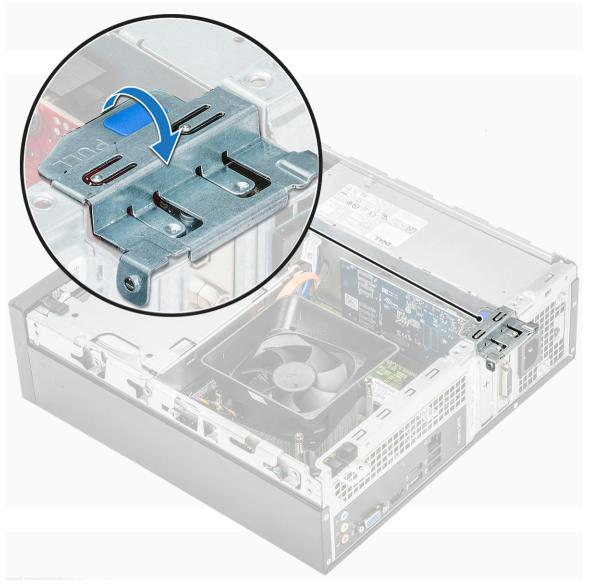
b Pull the card-retention tab [1], and remove the expansion card from the slot on the computer [2].
