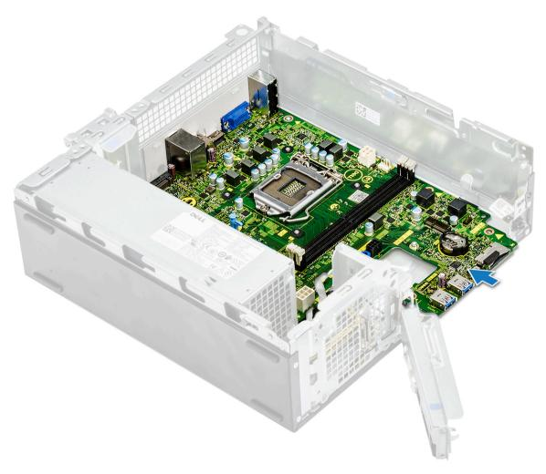
3 Replace the six 6-32xL6.35 screws to secure the system board.
