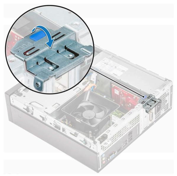
2 To remove the PCle bracket as shown below, insert a flathead screwdriver in the hole of PCle bracket [1], and repeatedly spin screwdriver from 0-45 degrees to release the bracket [2].
