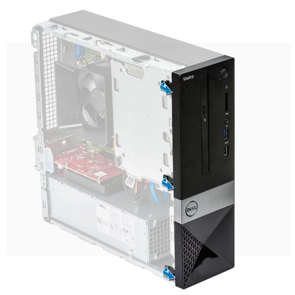
b Rotate the front bezel away from the computer [1] and pull to release the tabs on the front bezel from the front-panel slots [2].
