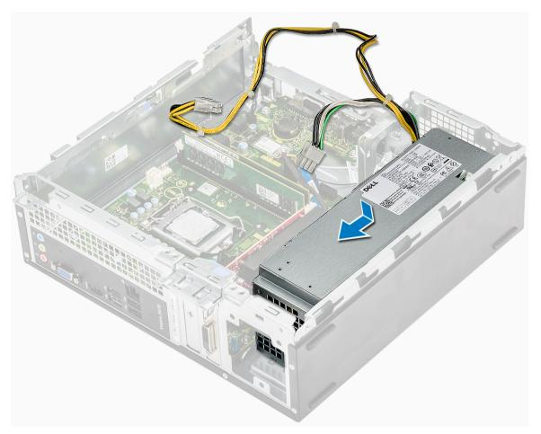
2 Replace the three 6-32xL6.35 screws to secure the power supply unit to the computer.
