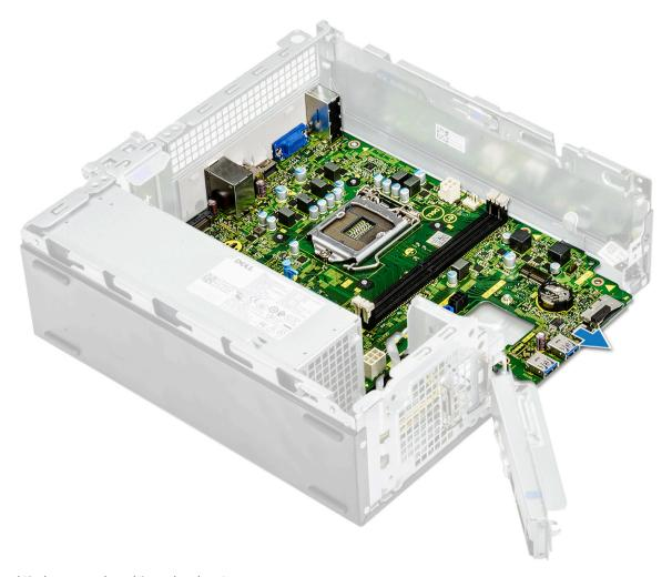
c Lift the system board from the chassis.
