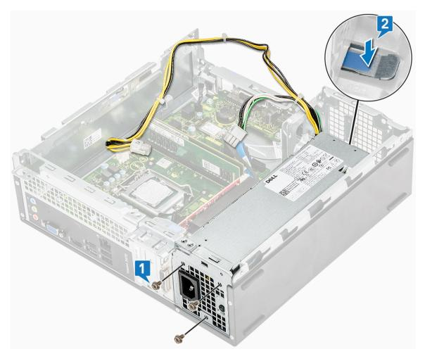
c Slide and lift the PSU from the computer.
