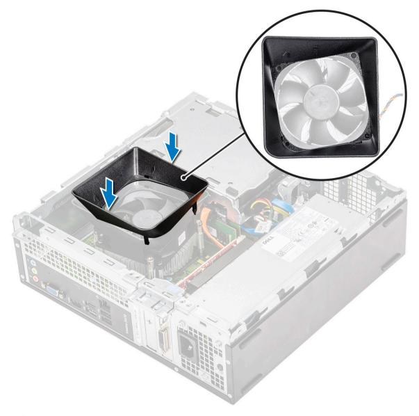
NOTE: Make sure the cooling shroud is placed such that the 'REAR' mark on the cooling shroud is towards the rear side of the system.
