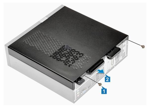
c Lift and remove the cover from the computer .
