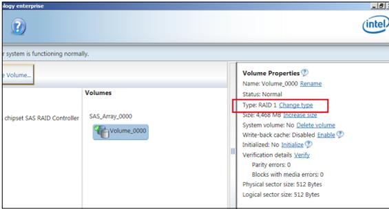
3. You can change the **Name**, **Select the new volume type**, and **Select additional disks to include in the new volume** if needed.
