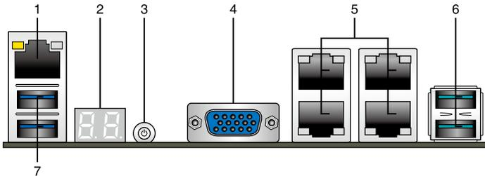
1. **RJ-45 port for iKVM.** This RJ-45 port functions only when you enable ASMB9 Management card.
