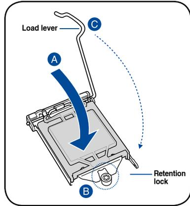
6. Insert the load lever under the retention tab to remove the PnP cap from the CPU socket.
