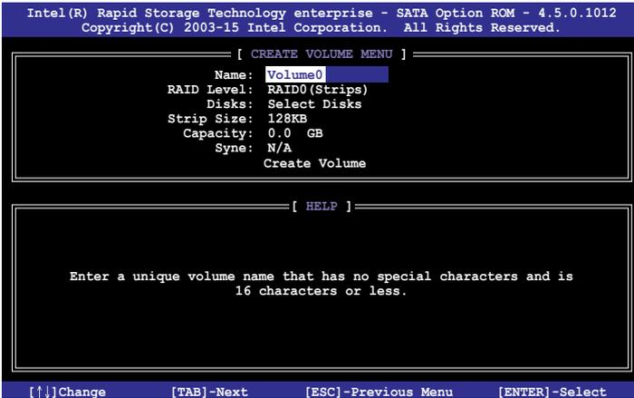
3. Press the up/down arrow keys to select a RAID Level that you wish to create then press <Enter>.
