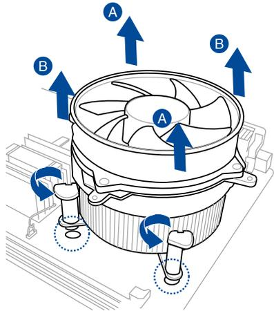
4. Carefully remove the heatsink and fan assembly from the motherboard.
