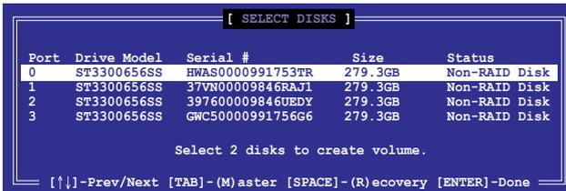
5. Use the up/down arrow keys to move the selection bar then press <Space> to select a disk. A small triangle before the Port number marks the selected drive. Press <Enter> when you are done.
