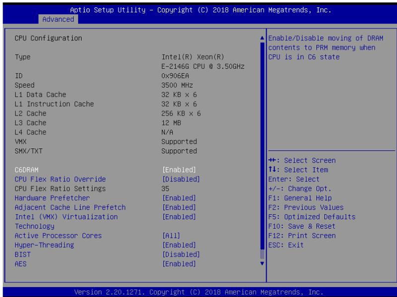
The screenshot shows the 'Advanced' tab of the Aptio Setup Utility. The 'CPU Configuration' section is expanded, showing various processor settings. The 'C6DRAM' option is highlighted in blue and is currently set to '[Enabled]'. A legend on the right side of the screen lists navigation keys: F1 for General Help, F2 for Previous Values, F5 for Optimized Defaults, F10 for Save & Reset, and F12 for Print Screen. The ESC key is used for Exit.
