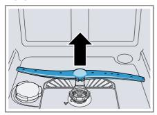
Check the outlet nozzles on the spray arms for blockages under running water and remove any foreign bodies.
