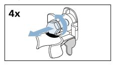
a) Remove the mains cable from the holders.
