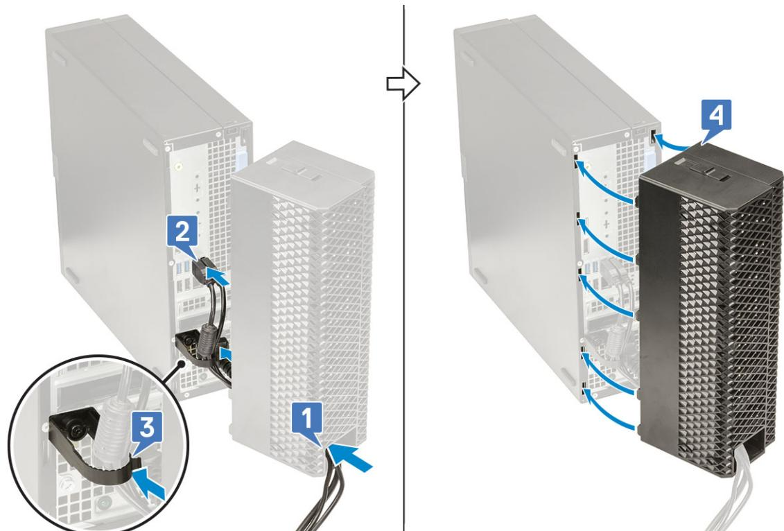
6 Gently press down on the cable cover until it clicks into place (1). Slide the latch towards the chassis (2) to lock the cable cover in place.
