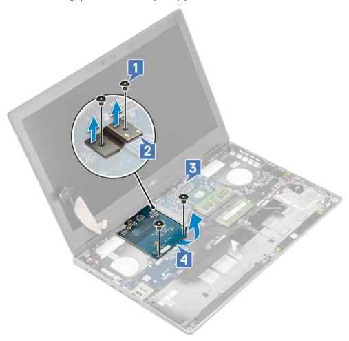
NOTE: The above procedures are for UMA graphics card. Systems shipped with UMA GPU card do not have GPU power cable. However, for discrete models shipped with either a 128 MB or 256 MB VRAM GPU card, you need to disconnect the GPU power cable before removing the GPU card.
