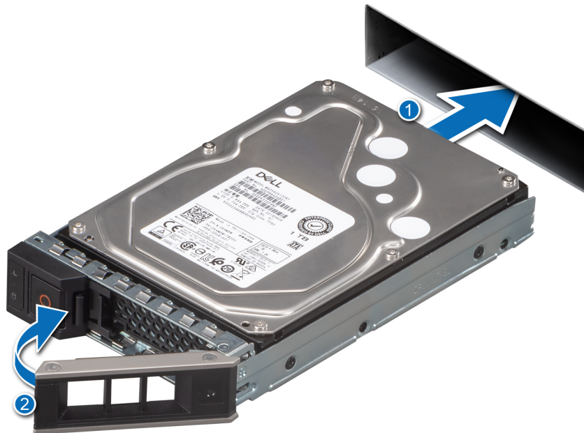
Figure 22. Installing the hot-swappable drive
