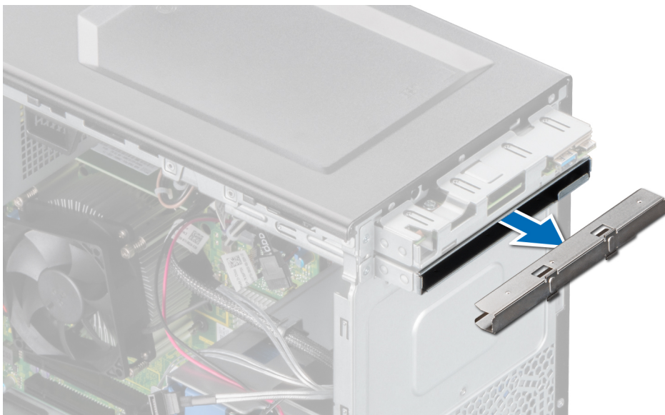
Figure 18. Removing the optical drive filler from the optical drive cage
