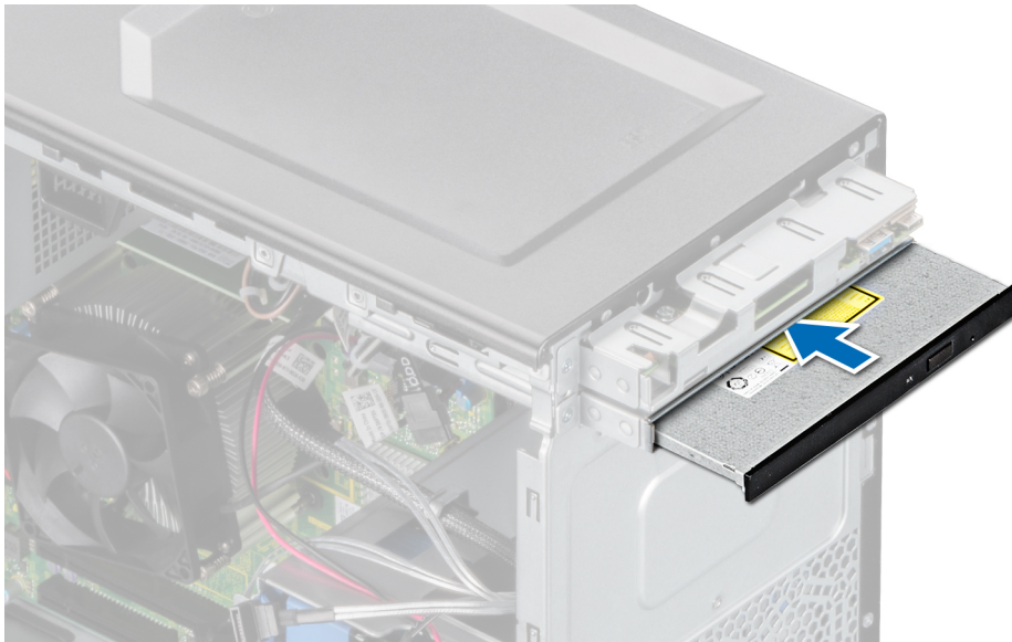
Figure 22. Installing the optical drive
