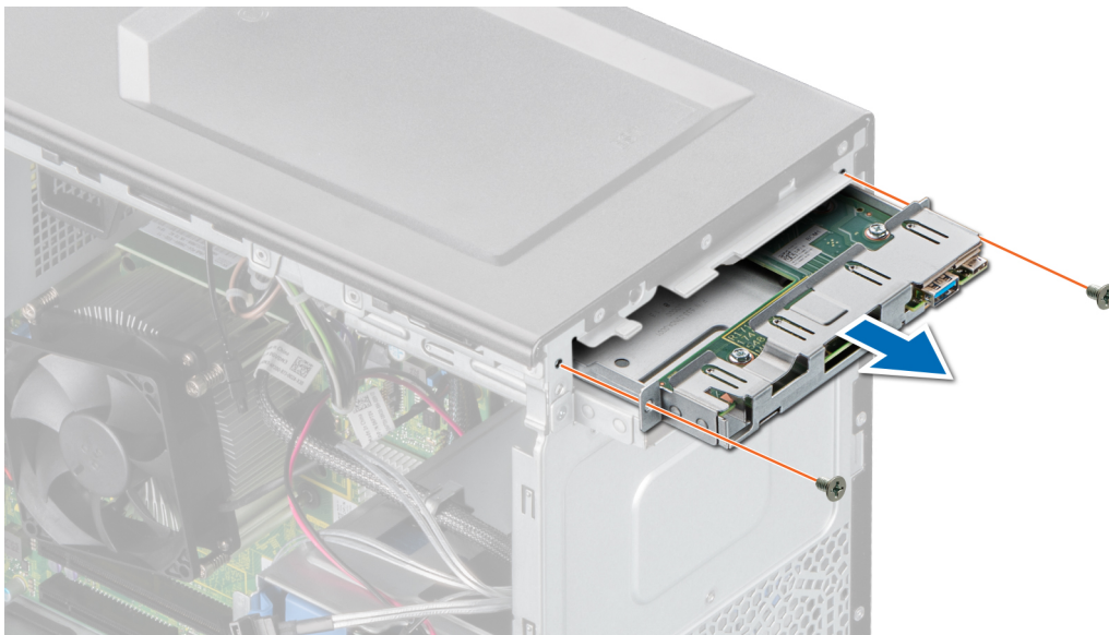
Figure 54. Removing the control panel cage
