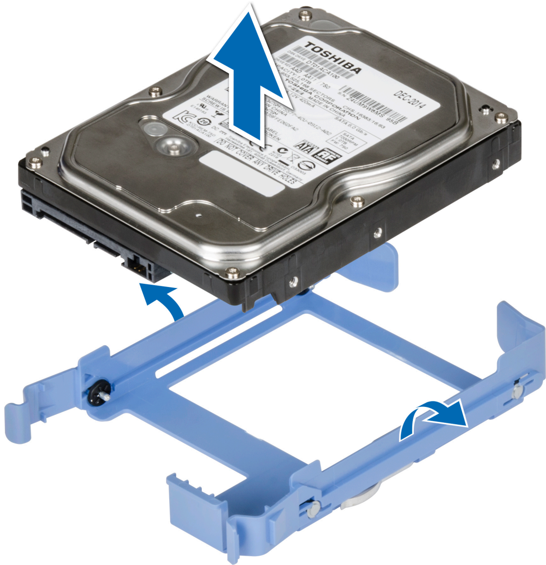
Figure 15. Removing the drive from the drive carrier
