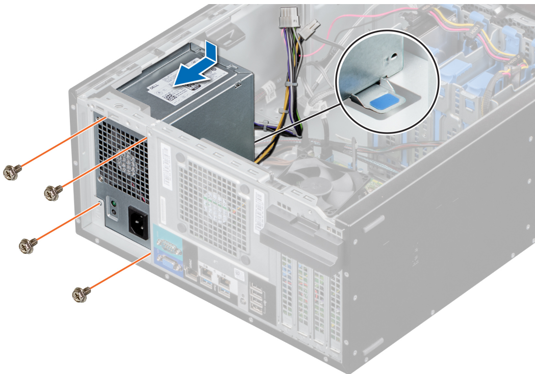
Figure 45. Installing the PSU
