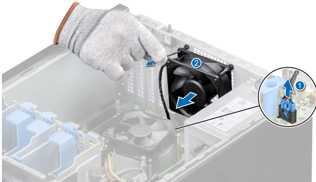
Figure 26. Removing the cooling fan
