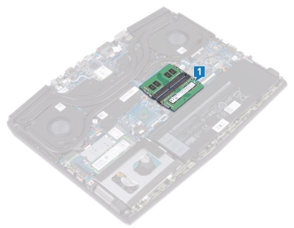
2 Use your fingertips to carefully spread apart the securing-clips on each end of the memory-module slot until the memory module pops up.
