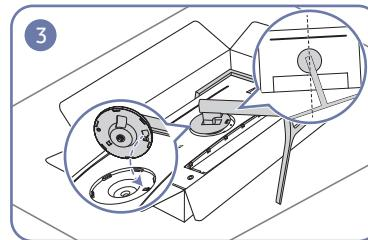
Place the stand neck of the display on the device as per the positions of the fasteners.
