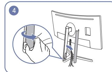
Open the COVER-STAND NECK LEFT, and rotate the open part at the bottom.
