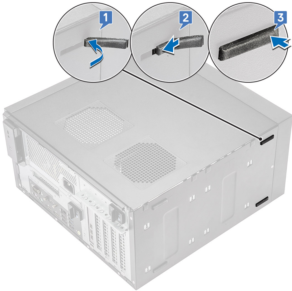
Figure 6. Front rubber feet installation
