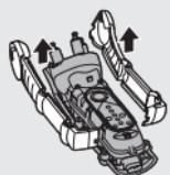
**4** Remove the side panels by pulling them off the sealed power unit.
