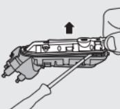
**7** Remove the back panel of the sealed power unit by means of a screwdriver.
