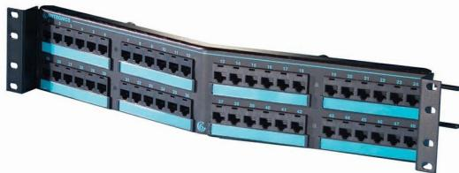
Clarity® SNAPT™ patch panels offer improved rear cable management with the addition of an adjustable depth rear management bar. The rear portion of these bars is also removable to provide more working room for the initial termination of panels. After cables are SNAP terminated, the rear bars are attached and adjusted to the depth that best matches the cable and rack selections.
