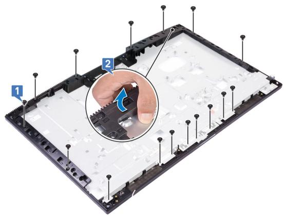
5 Lift the middle frame off the display assembly base [1].
