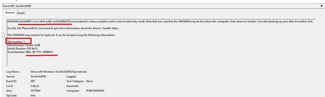
Figure 23. Operational and Diagnostics Logging information: NVDIMM-N Disk
