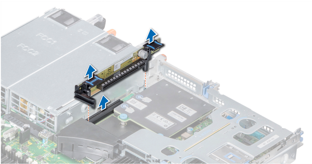
Figure 48. Removing the expansion riser 2A
