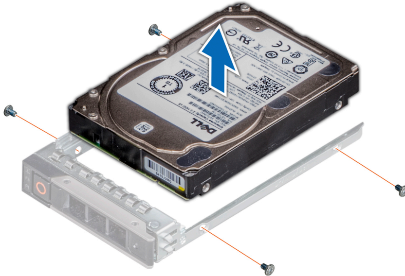
Figure 77. Removing the drive from the drive carrier
