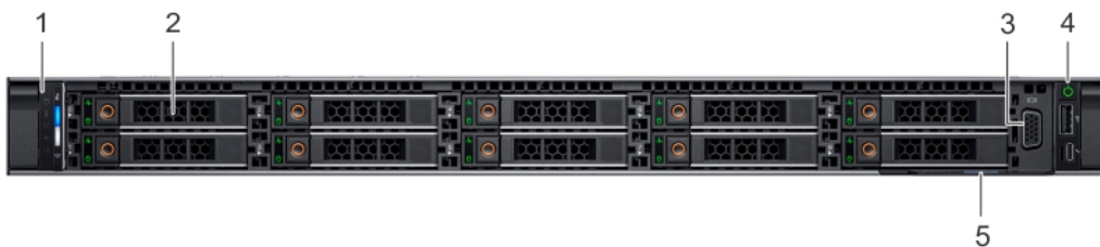
Figure 4. Front view of 10 x 2.5-inch drive system
