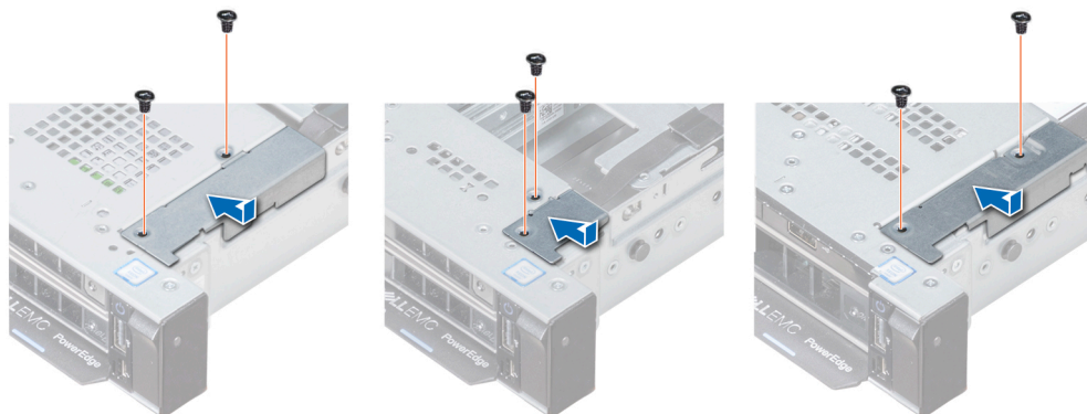
Figure 118. Installing the cable cover
