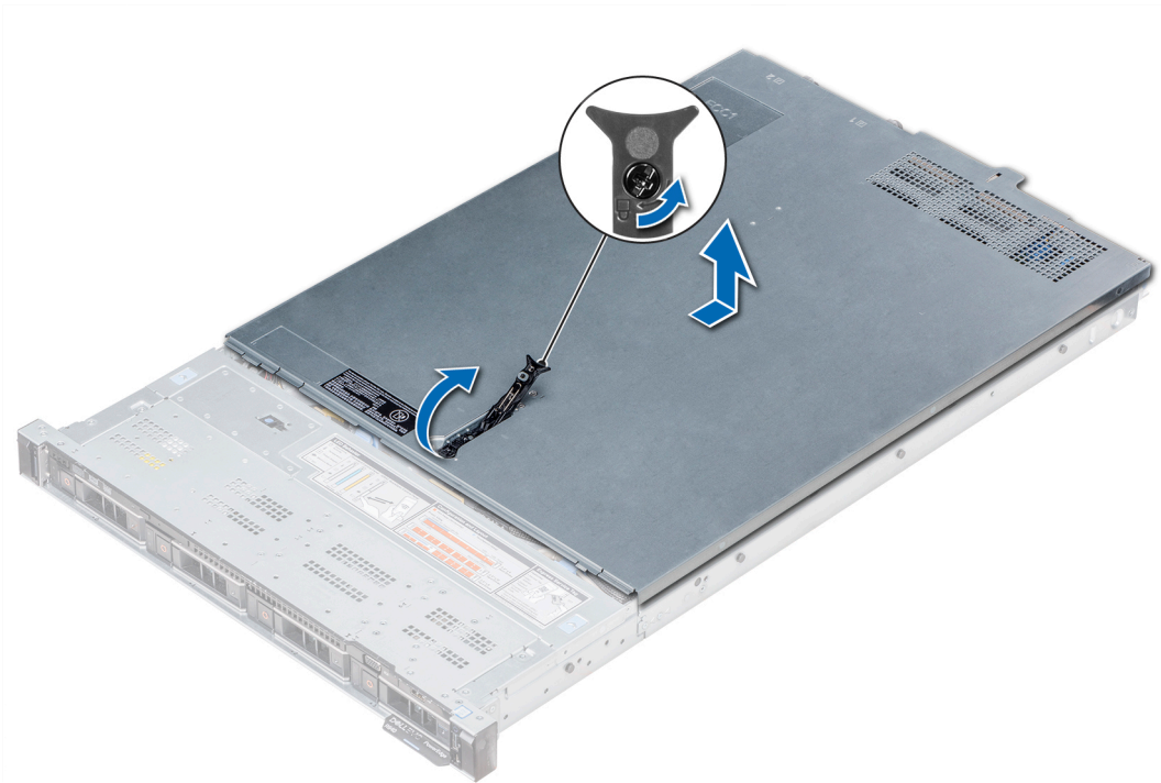
Figure 22. Removing the system cover
