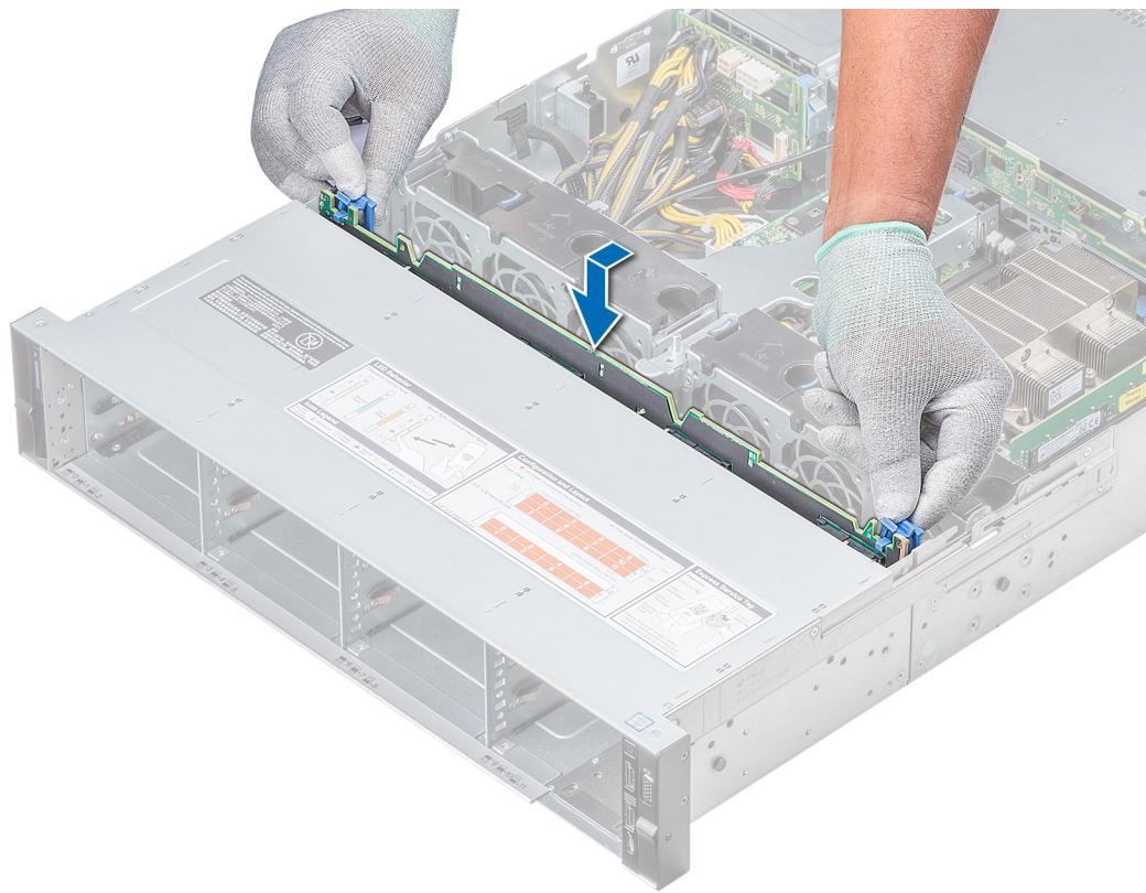
Figure 100. Installing the backplane
