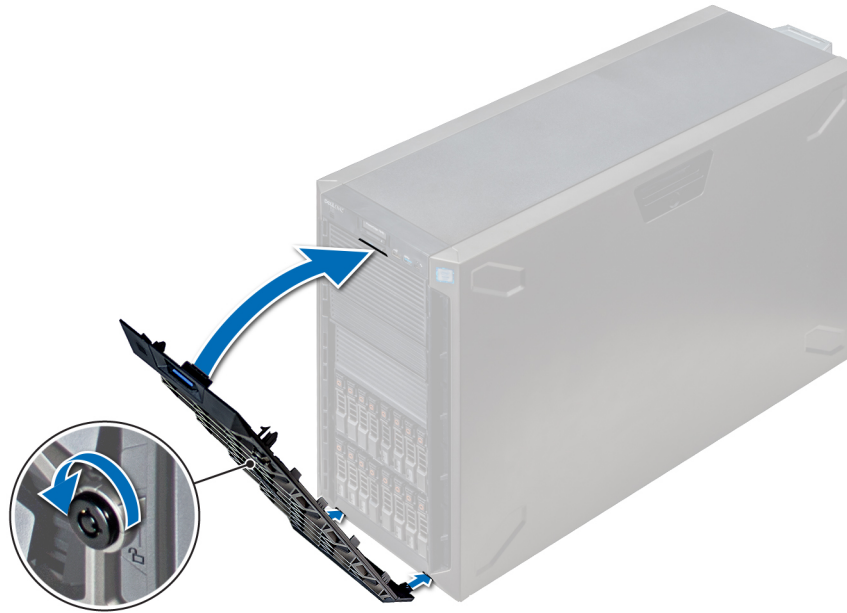
Figure 22. Installing the front bezel
