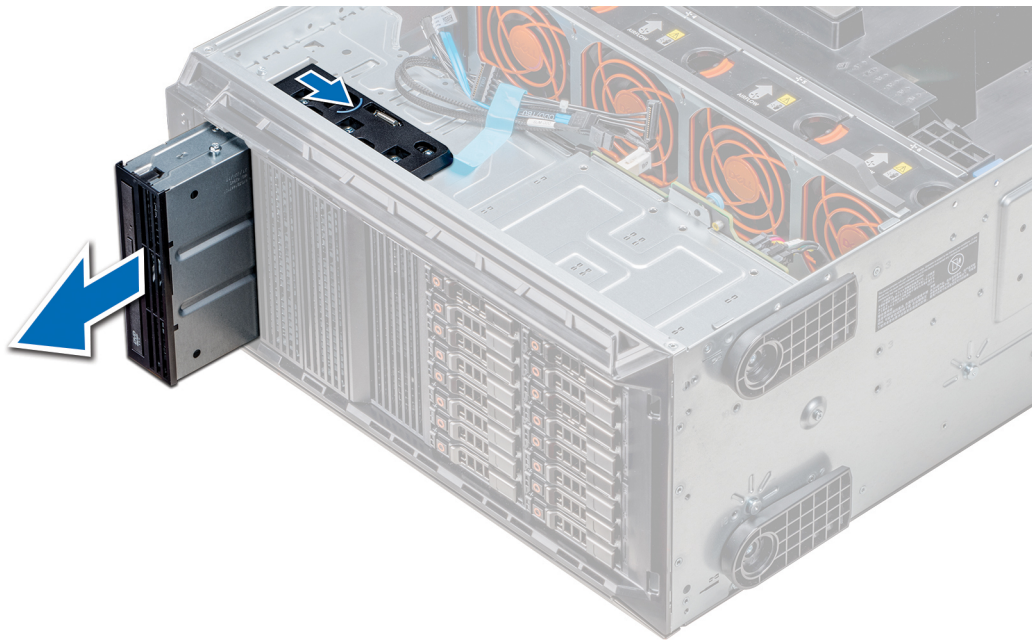
Figure 57. Removing the optical drive cage or tape drive
