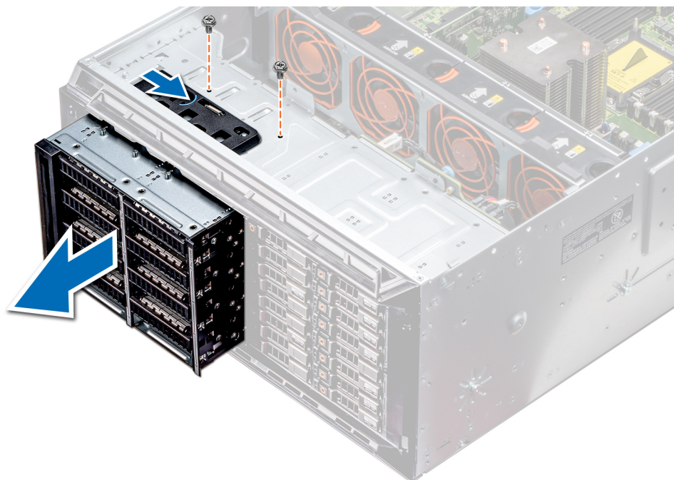
Figure 53. Removing a NVMe drive bay or flex bay
