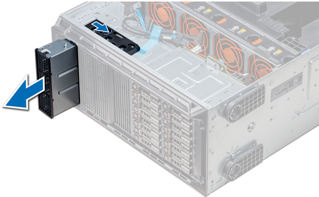
Figure 55. Removing the optical drive or tape drive
