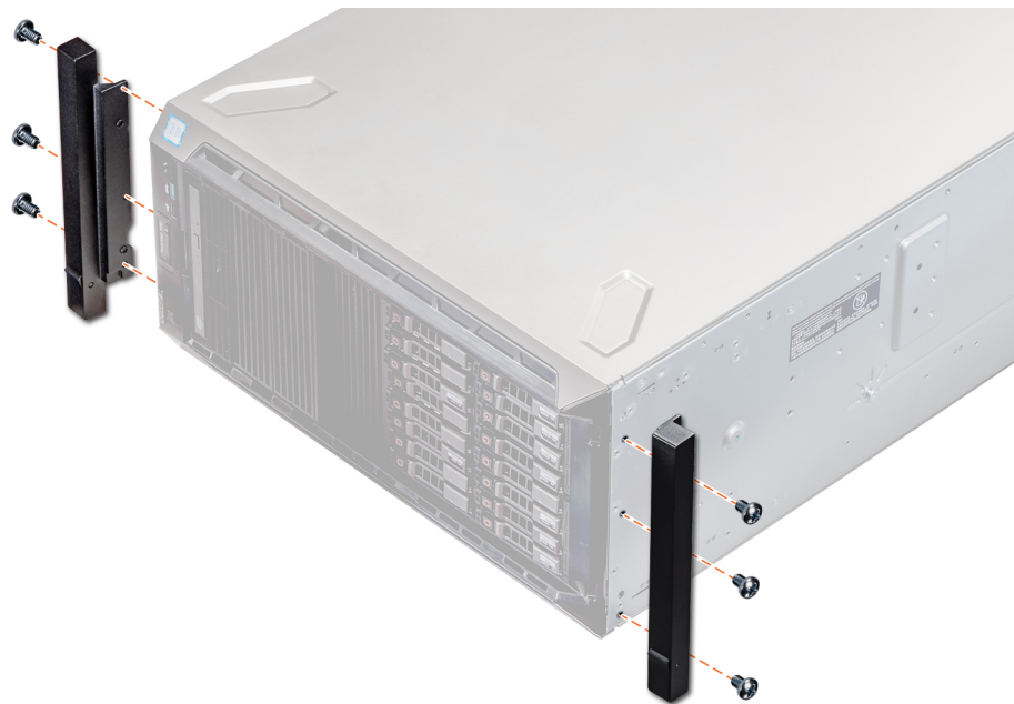
Figure 116. Installing the system ears
