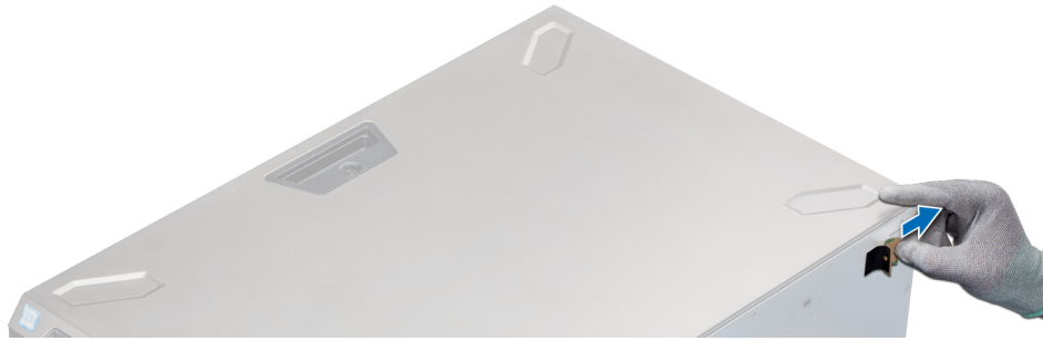
Figure 115. Attaching the mylar cover
