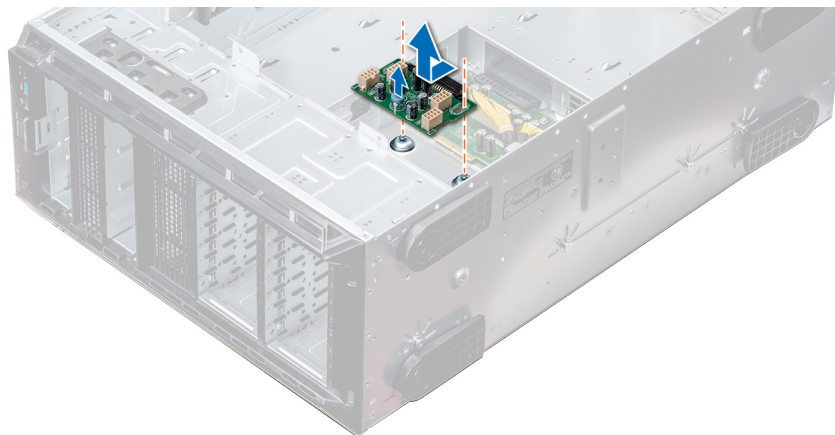
Figure 110. Removing the GPU power interposer board
