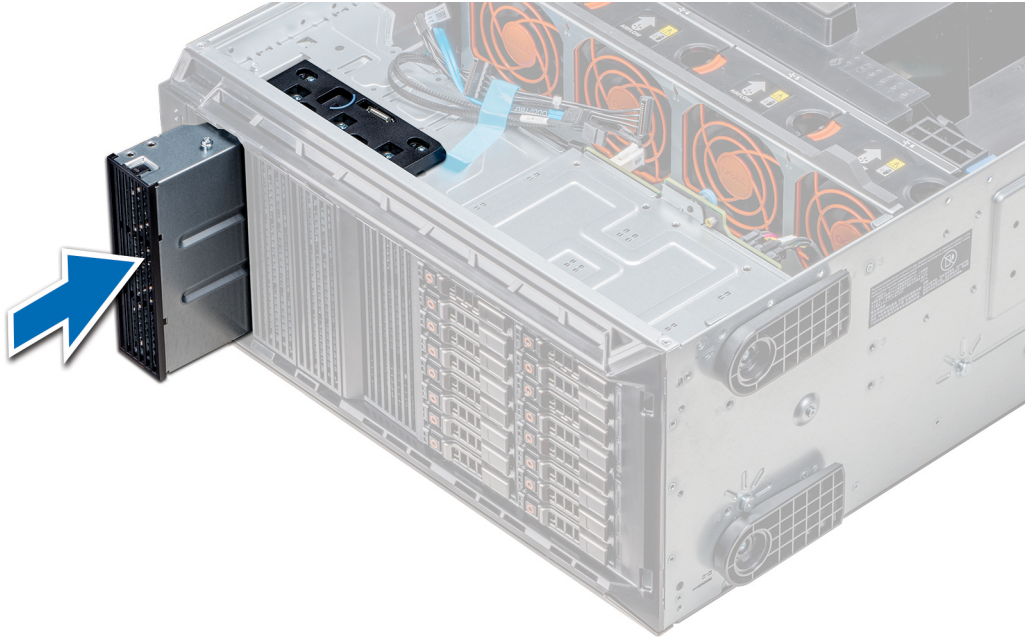
Figure 56. Installing the optical or tape drive blank
