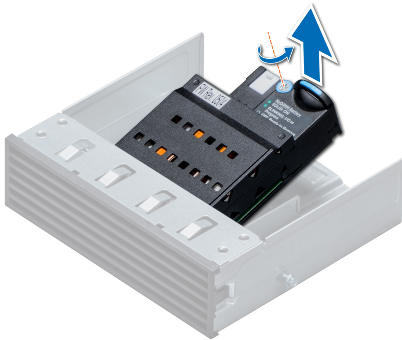
Figure 61. Removing the NVDIMM-N battery
