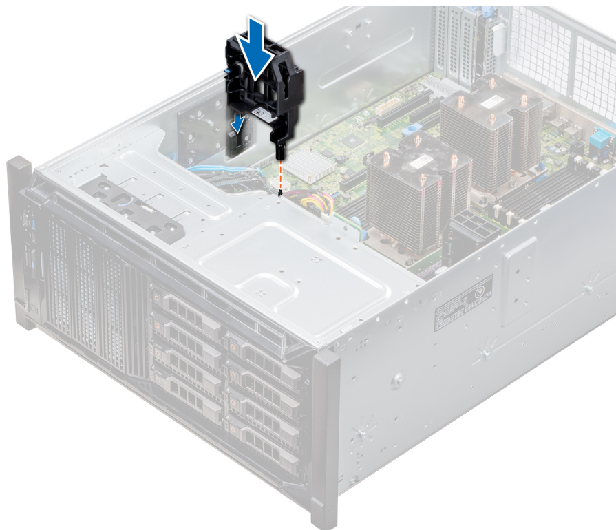
Figure 68. Installation du support de carte GPU
