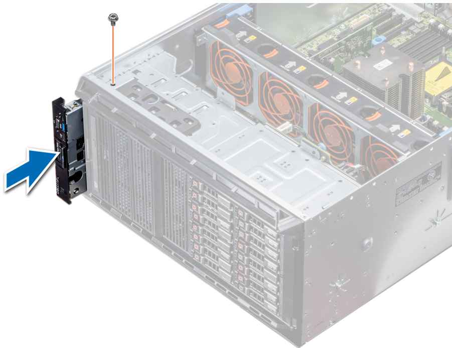
Figure 103. Installing the control panel assembly
