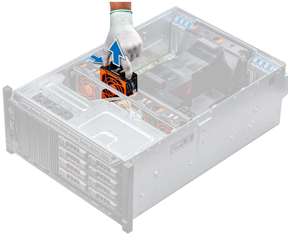
Figure 47. Removing a middle cooling fan
