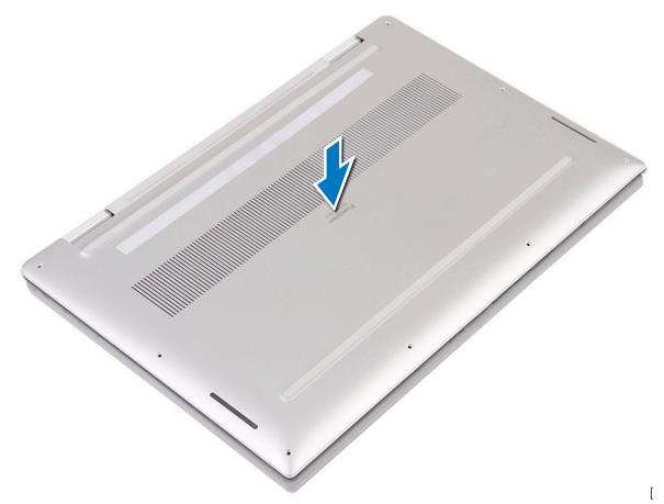
3 Snap the base cover into the tabs on the palm-rest and keyboard assembly [1, 2].
