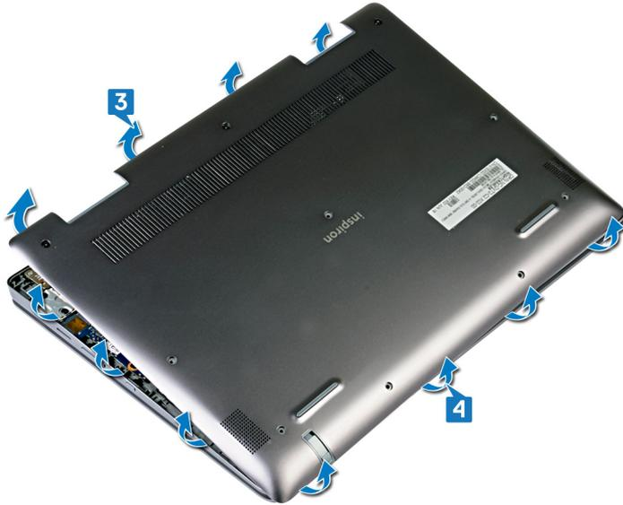
4 Remove the base cover carefully off the palm-rest and keyboard assembly.
