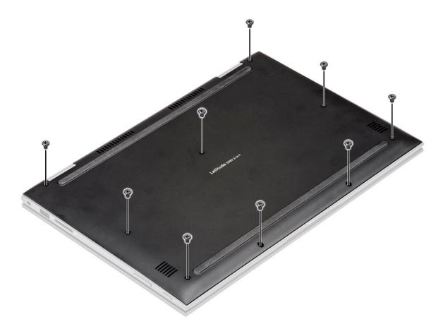
4 Using a plastic scribe, pry the base cover from the edges of the laptop chassis [1].
