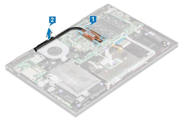
(i) NOTE: Loosen the captive screws using a diagonal or crisscross pattern as printed on Heatsink. The screws are captive screws and cannot be fully removed.
