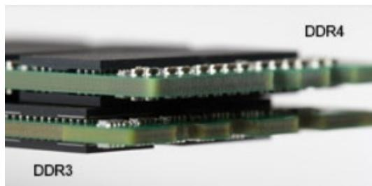
**Figure 2. Thickness difference**
