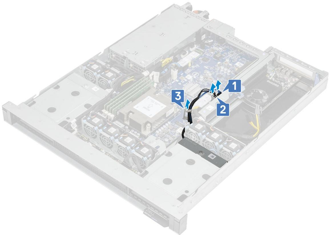
a Loosen the one captive screw [1], lift the HDD backplane away from the system chassis [2].
