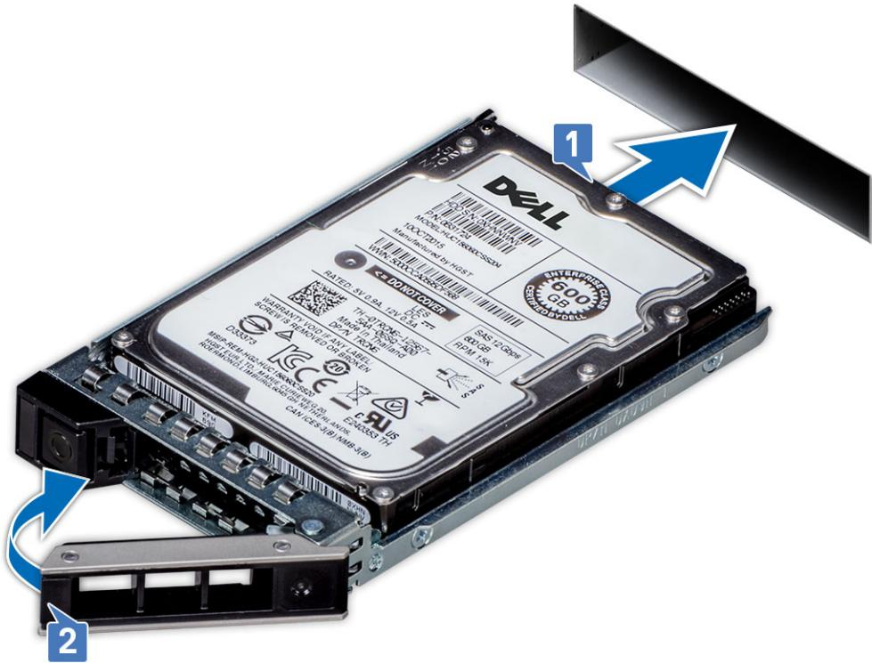
**NOTE:** Ensure that the release latch [2], is open while inserting the had drive back into the slot.
