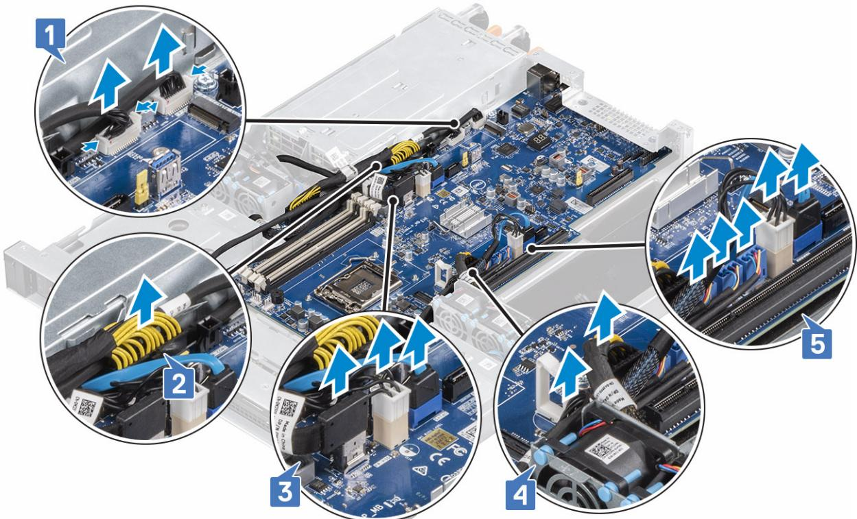
4 To remove the system board screws and system board:
