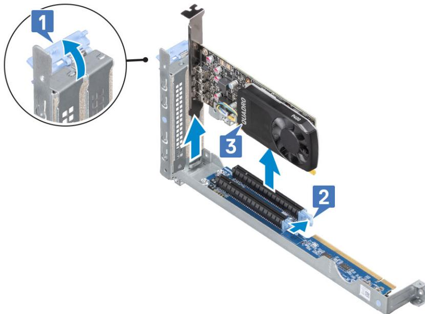
**NOTE:** If removing the graphics card permanently, install Riser1 blank in empty expansion slot opening.
