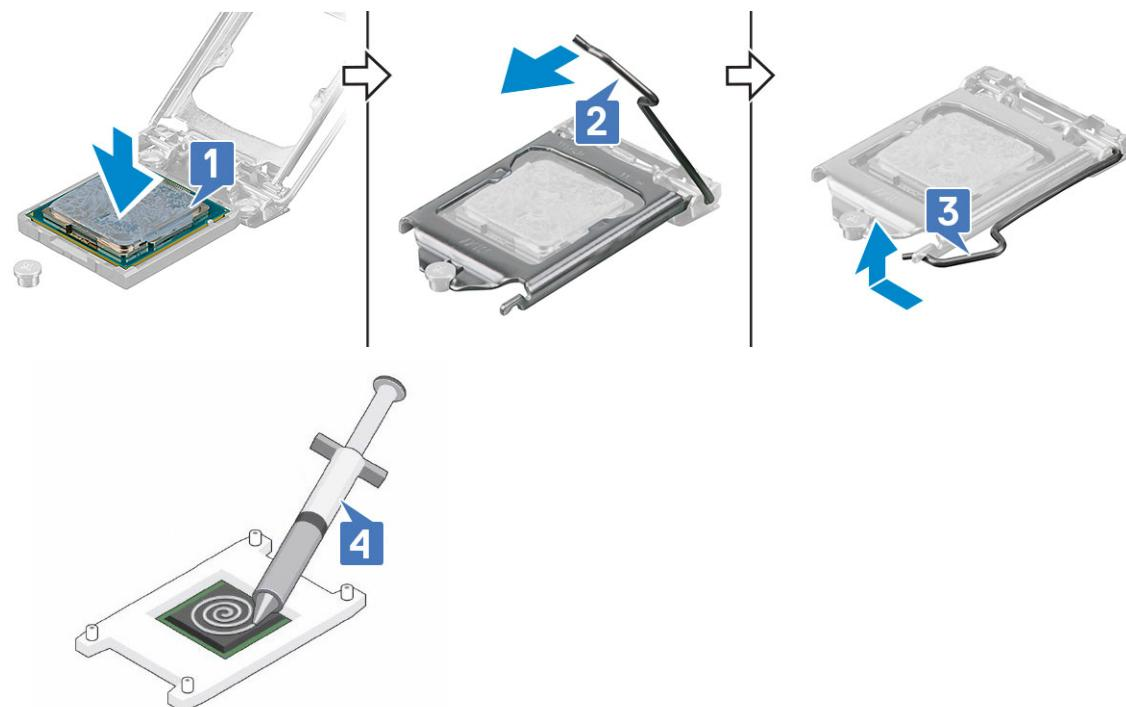
**NOTE:** The thermal-grease is intended for one-time use only. Dispose of the syringe after you use it.
