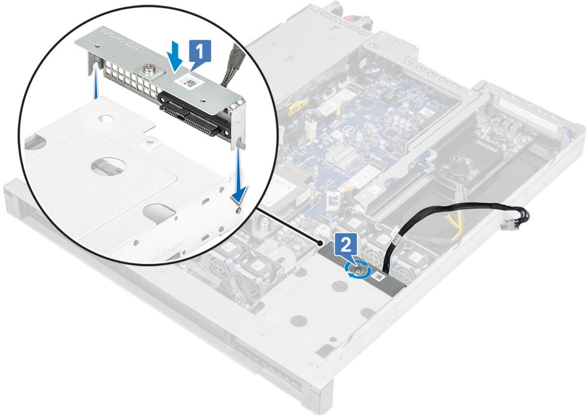
**NOTE:** The hard drive back plane slots need to align with the alignment pins on the hard drive cage.
