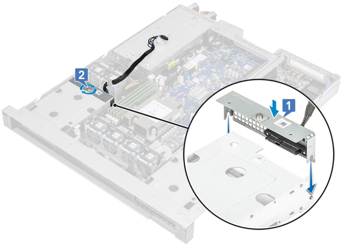
**NOTE:** The hard drive back plane slots need to align with the alignment pin on the hard drive cage.
