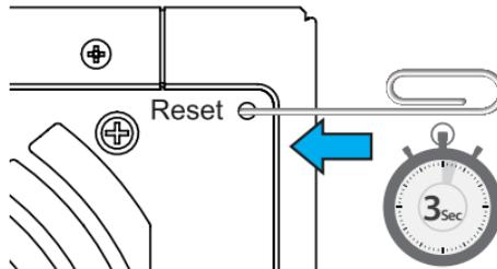
To revert to the default password, use a pin to press the Reset button for three seconds or until you hear a short beep - - - - - en
