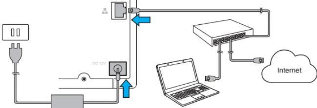
Plug the network cable into the NAS, and into a switch or router
