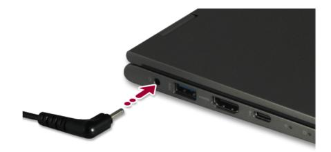
2 Open the LCD and check the charging state. When the AC adapter lamp is blinking, charge it fully with the AC adapter before using it.
