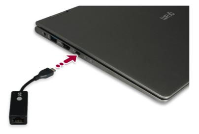
2 Connect the wired LAN cable to the LAN port.
