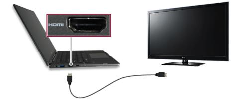
3 On the PC, press [Fn] + [F7] to display monitor (projector) toggling screen. Select the desired screen output.
