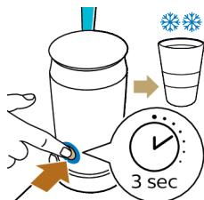
Note: Press the button for 3 seconds for cold frothed milk.
