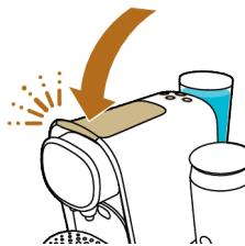
6 Place a bowl with a minimum capacity of 1.5 liters on the lower drip tray under the coffee dispensing spout to collect the descaling solution.
