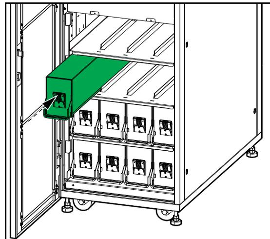
3. Fasten the batteries with a screw on the front of the battery.
