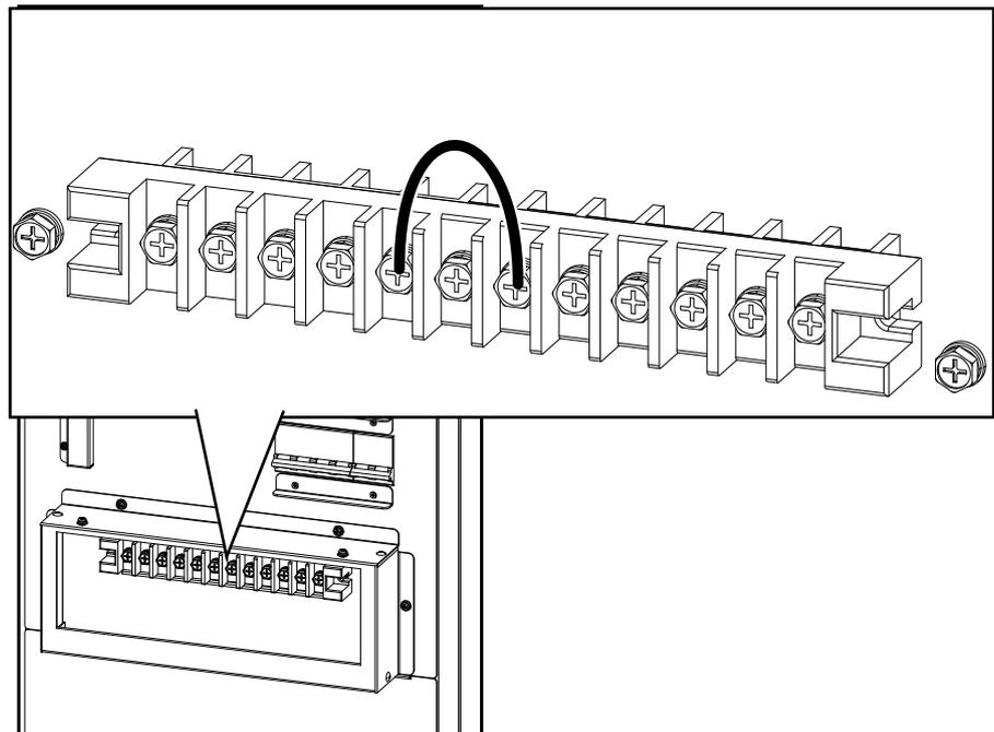
4. Route the power cables through the bottom of the conduit box.
