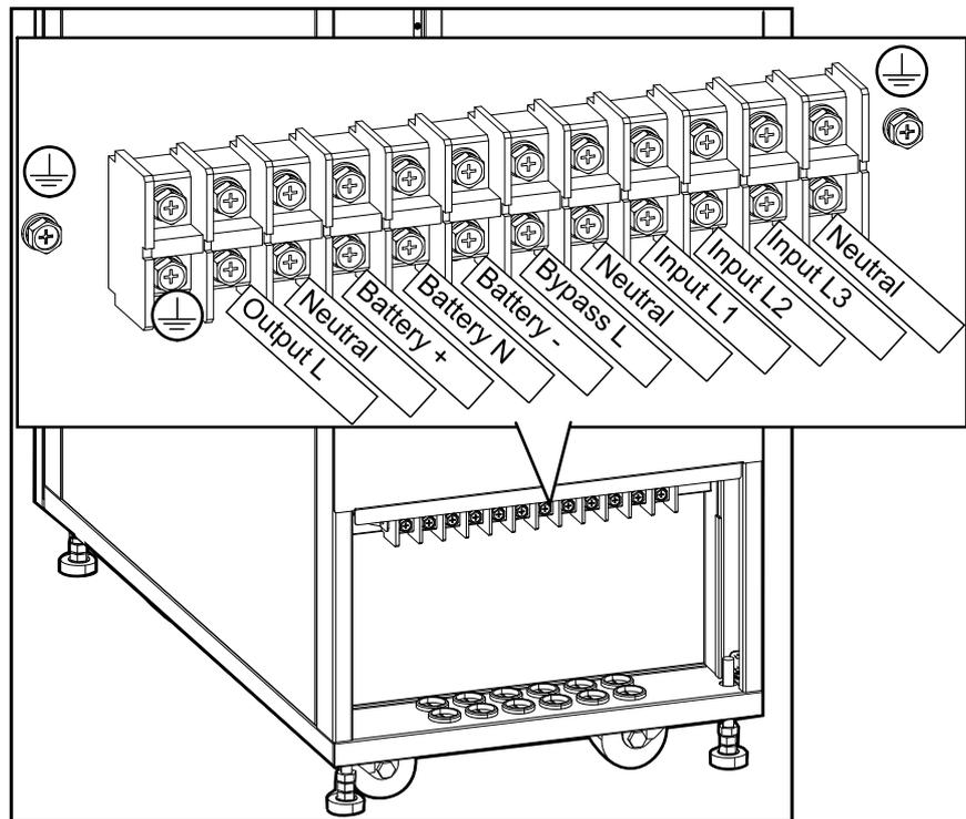
6. Connect the input cables, output cables, and bypass cables (if applicable).
