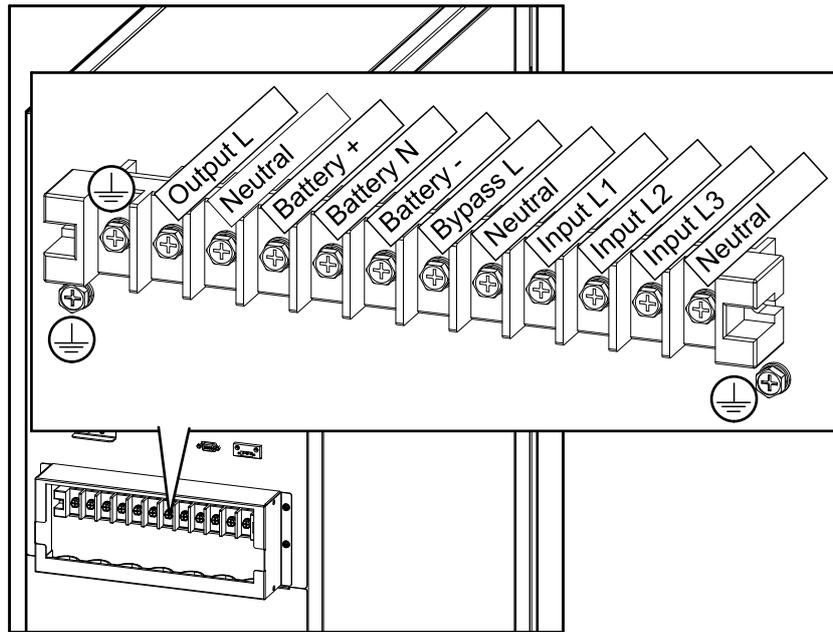
6. Connect the input cables, output cables, and bypass cables (if applicable).
