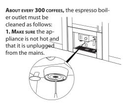
**2. Using a screwdriver,** unscrew the screw fixing the espresso boiler outlet filter
