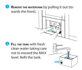
Never use the appliance without water in a the tank and always remember to top up when the level drops to a couple of centimetres from the bottom.
