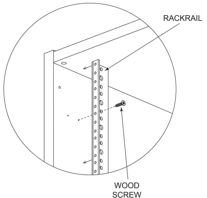
**NOTE:** When moving front rackrail to setback position, mount rail to recessed pilot holes on opposite end of side panel. This hides the original mounting holes from view.
