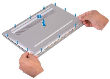
2 Replace the eight screws (M2x3, Torx) that secure the base cover to the palm-rest assembly.
