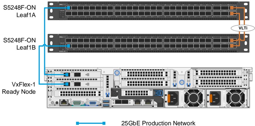
Figure 7 VxFlex-1 wiring to production network
