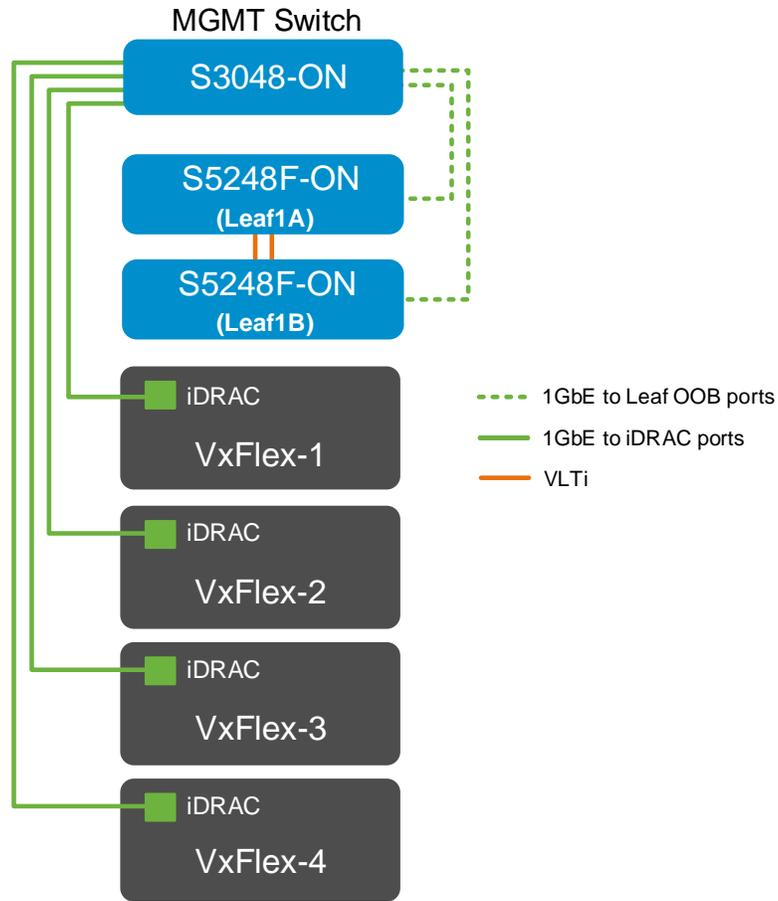
Figure 6 Management network for a single rack
