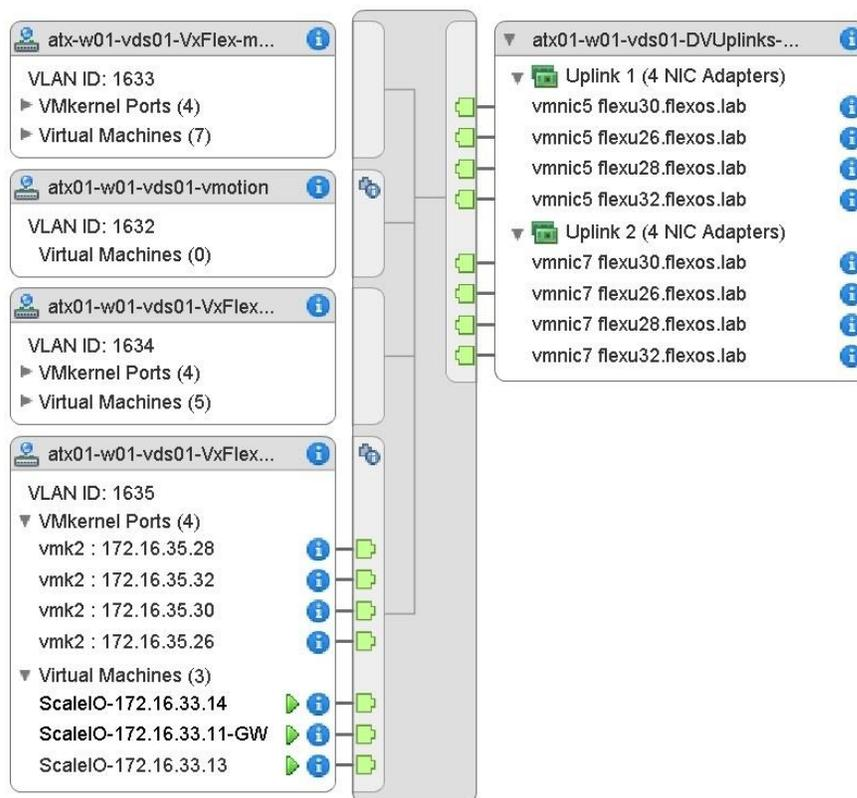
Figure 9 VDS atx01-w01-vds01 topology shown in vCenter
