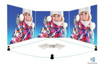
IPS displays use advanced technology that gives you extra-wide viewing angles of 178/178 degrees, making it possible to view the display from almost any angle — even in 90-degree Pivot mode! Unlike standard TN panels, IPS displays gives you remarkably crisp images with
