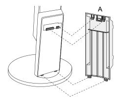
2. Slide (A) downward to secure the tabs to the attachment parts of the stand.
