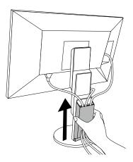
2. While holding down  $\equiv$  of (A) lightly, slide (A) upward to detach it from the stand.
