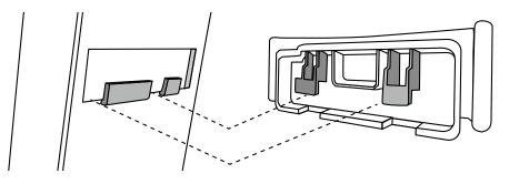
2. Slide the cable holder to the right, and attach it to the stand.
