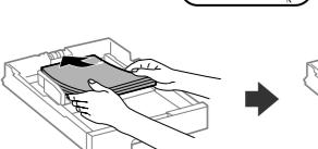
Load A4 size paper toward the back of the paper cassette with the printable side face down then slide the front edge guide to the paper.
