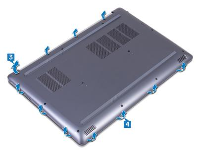
5 Pry the base cover from the right side and lift it off the palm rest and keyboard assembly.
