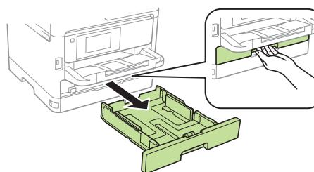
**2** Slide the side edge guides all the way out and set the front edge guide to the paper size you are using.
