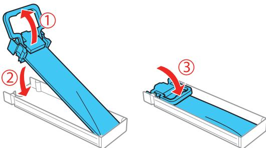
**Note:** Make sure the ink pack is fully inserted and level with the top of the ink pack tray.
