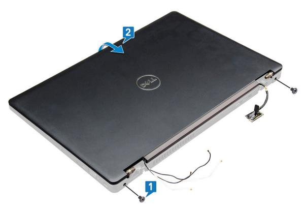
7 Slide the display assembly away from the system base.
