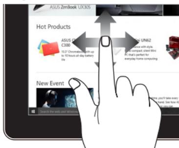
Slide your finger to scroll up and down and slide your finger to pan the screen left or right.
