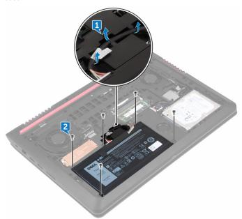
Using the pull tab, lift the battery, along with its cable, off the computer base.
