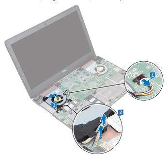
Disconnect the right-fan cable from the system board.
