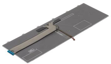
**2** Gently fold the keyboard-backlight cable till the edge of the keyboard cable as shown in the image.
