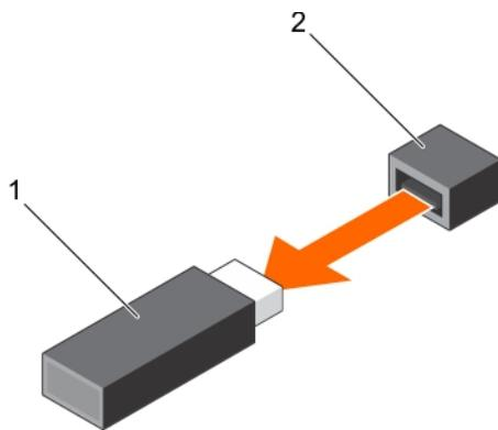
**Figure 50. Removing the internal USB memory key**
