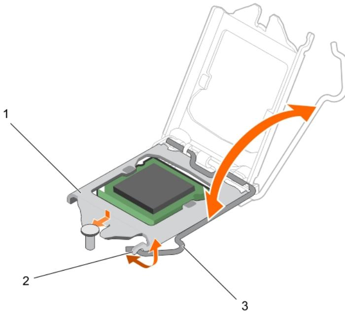
**Figure 65. Opening and closing the processor shield**
