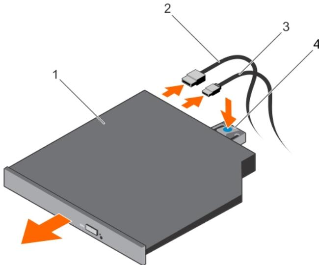
**Figure 44. Removing the optical drive**
