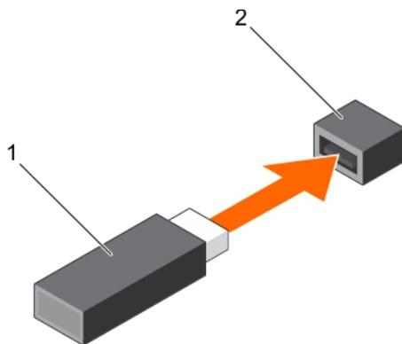
**Figure 51. Installing the internal USB memory key**
