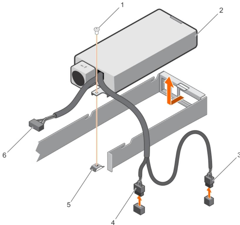
**Figure 68. Removing a cabled power supply unit**
