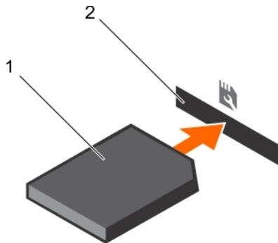
**Figure 59. Installing an optional SD vFlash card**
