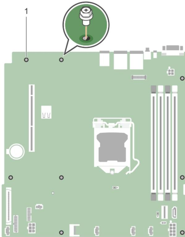
**Figure 83. Removing the screws on the system board**
