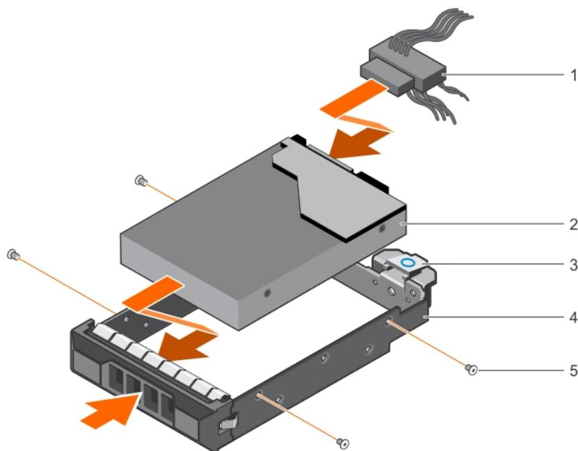
**Figure 31. Installing a cabled hard drive carrier**
