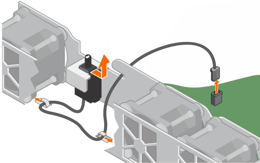
**Figure 19. Removing the intrusion switch**
