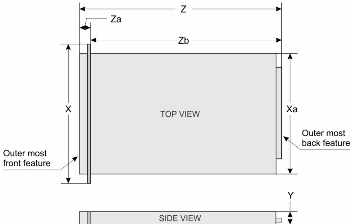
Figure 11. Chassis dimensions of the PowerEdge R230 system
