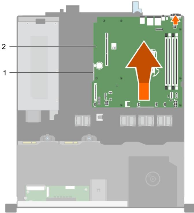
**Figure 85. Install the system board**
