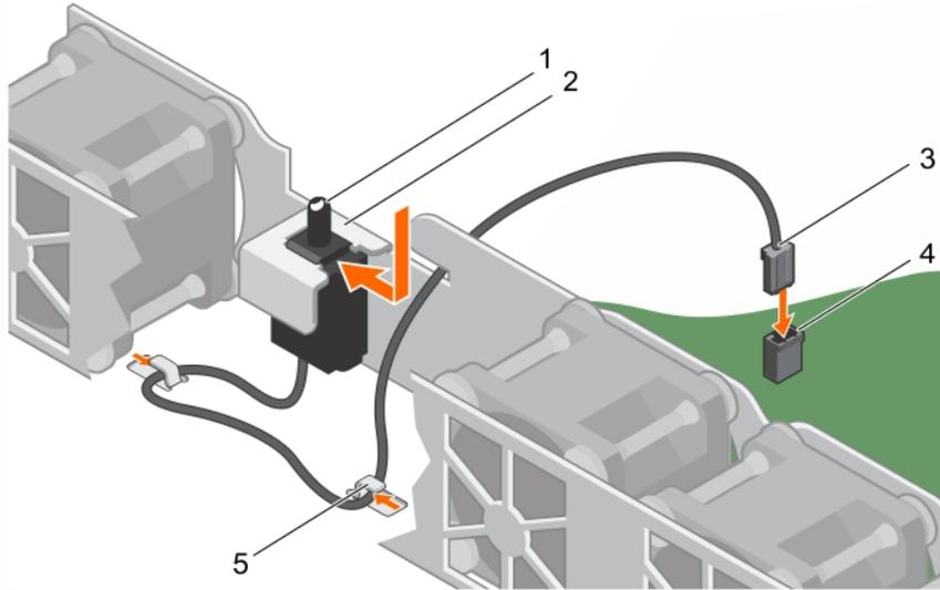
**Figure 20. Installing the intrusion switch**
