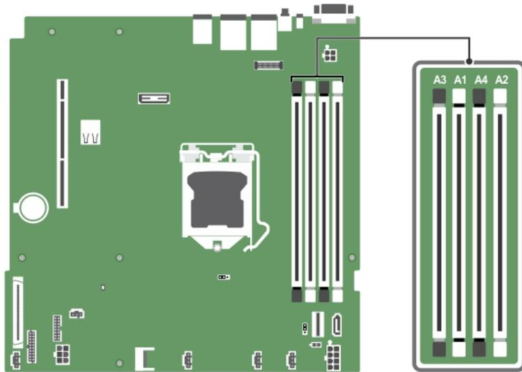
**Figure 23. Memory socket locations on the system board**
