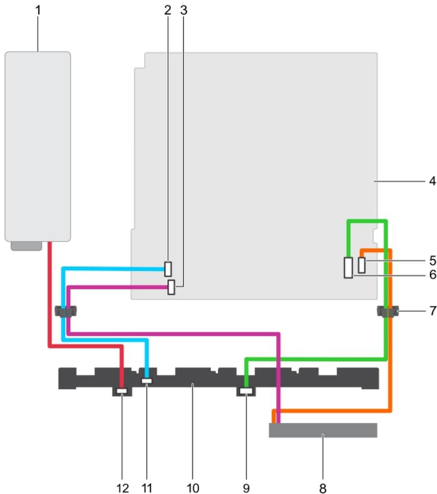
**Figure 73. Cabling diagram—Four 3.5-inch hot swappable SAS/SATA hard drive backplane**
