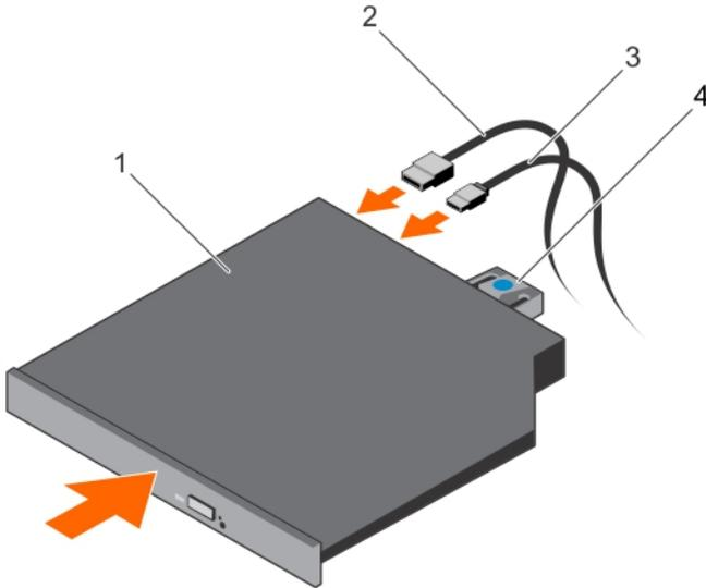
**Figure 45. Installing the optical drive**
