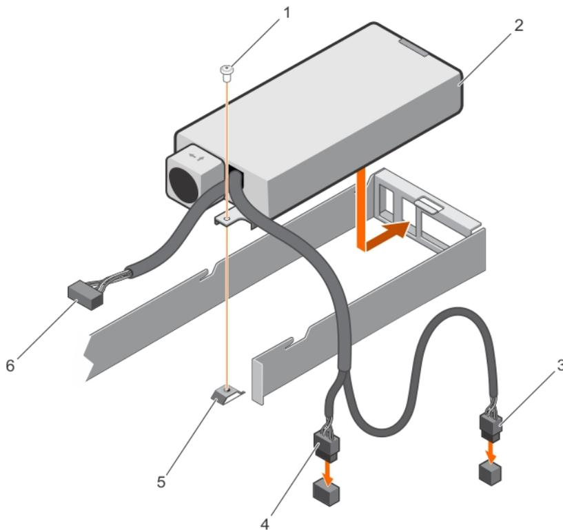
**Figure 69. Installing a cabled PSU**
