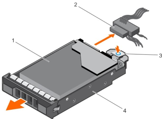
**Figure 28. Removing a cabled hard drive carrier**
