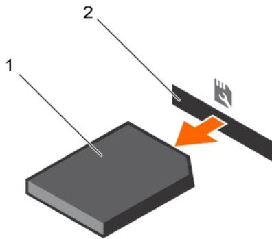
**Figure 58. Removing the optional SD vFlash card**
