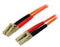
The 50FIBLCLC10 10m LSZH LC to LC Fiber Cable features 50/125 micron fiber for high-speed, high bandwidth data transmissions over Gigabit Ethernet and Fiber Channel networks, with support for duplex multimode applications.
