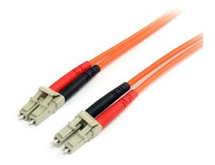
The FIBLCLC10 10-meter (32.8ft) Multimode 62.5/125 Duplex Fiber Patch Cable is terminated at both ends with LC (male) connectors, to provide the necessary connection between fiber networking devices for high-speed, long distance networks.
