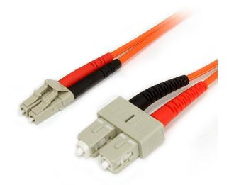
The FIBLCSC1 1-meter (3.2ft) Multimode 62.5/125 Duplex Fiber Patch Cable is terminated with one LC (male) connector and one SC (male) connector, to provide the necessary connection between fiber networking devices for high-speed, long distance networks.
