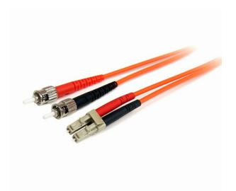
The FIBLCST7, 7-meter (23ft) Multimode 62.5/125 Duplex Fiber Patch Cable is terminated with one LC (male) connector and one ST (male) connector, to provide the necessary connection between fiber networking devices for high-speed, long distance networks.
