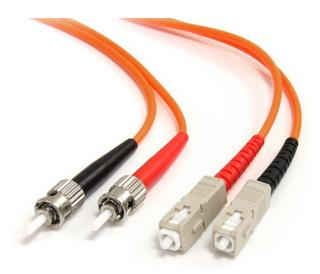
The FIBSTSC1, 1-meter (3.3ft) Multimode 62.5/125 Duplex Fiber Patch Cable is terminated with one ST (male) connector and one SC (male) connector, to provide the necessary connection between fiber networking devices for high-speed, long distance networks.
