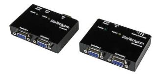
The ST121UTPGB VGA Video Extender over Cat5 allows you to extend your VGA video signal by up to 150 meters (500 feet) and connect up to 4 displays (2 local and 2 remote) from that single source. The ST121UTPGB is a bundled kit including both a local transmitter and a remote receiver unit, offering a complete solution for scenarios in which remote monitor displays are required.
