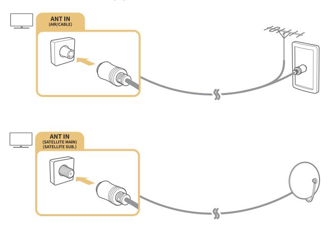
It is best to connect the both connectors using a Multi-Switch or DiSEqC Switch, etc and to set **Aerial Connection Type** to **Dual**.
