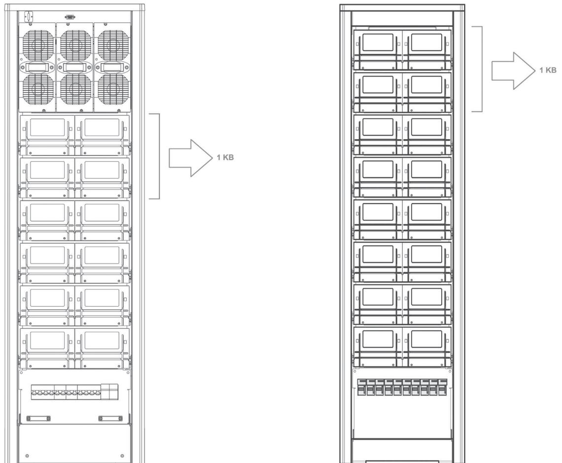
It is necessary to install 1 KB every 10 kVA of nominal UPS power in case of modular cabinets with battery drawers.
