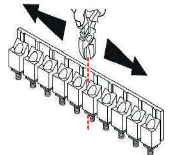
2. Eliminate the vertical connections that are not represented in the connection diagrams.
