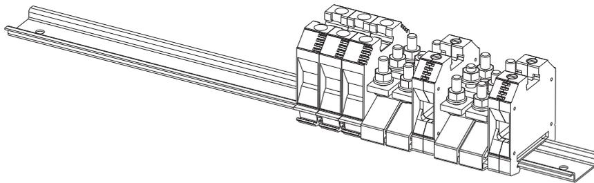
3. Remove the central metal rod between the two positive poles +0 and +1.
