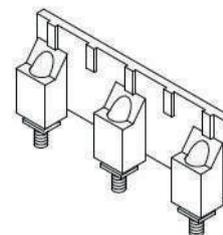
4. Carefully tighten all the screws to the terminal strip.
