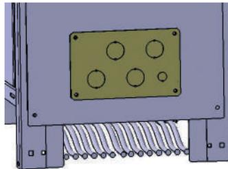
In the case of the Trimod HE 80 kVA, the cables must be passed into the opening at the base. The fastening is done on the appropriate bar by means of clamps and clips present in one of the accessory packs.
