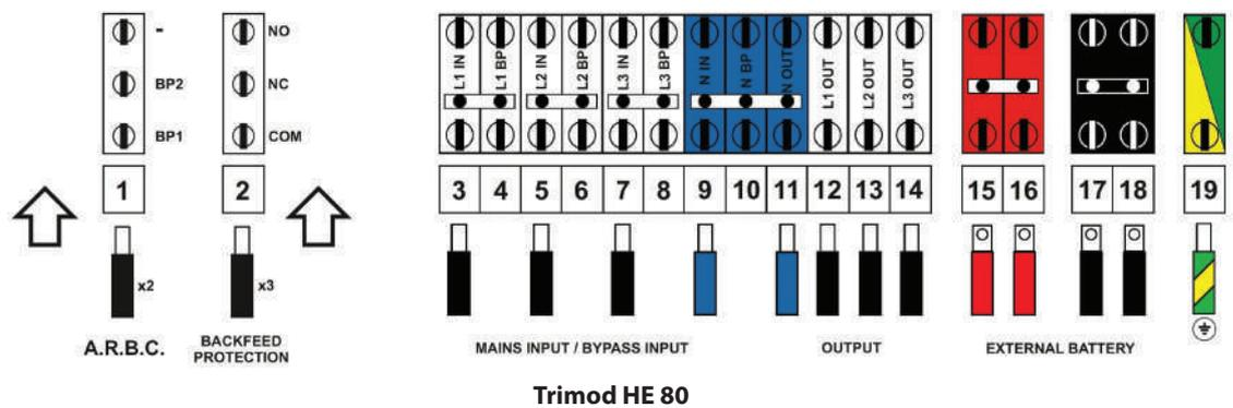
4.3.2 THREE PHASE input - THREE PHASE output connection with separate bypass input line
