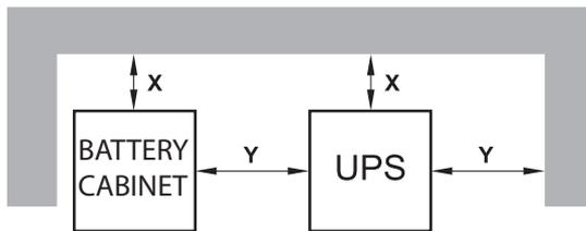
The UPS must be positioned respecting the following conditions:
