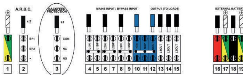
If the UPS detects a voltage backfeed, the relay is energised and changes status, enabling the disconnection of the input lines that must be done externally as indicated in the diagrams shown below.
