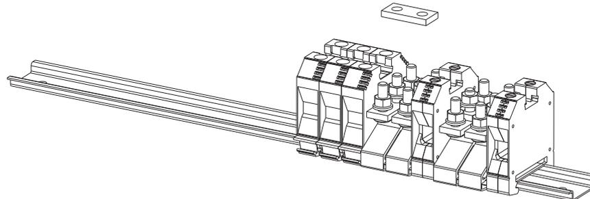
4. Separate the positive terminals +0 and +1 and insert the insulating functional separator supplied in the accessory kit into the DIN rail.
