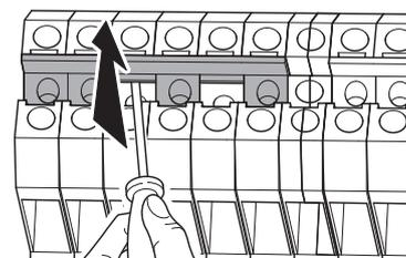
7. Check that the screw head abuts properly on the terminals.
