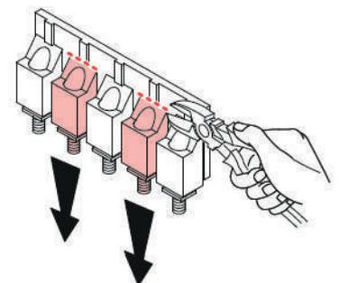
3. Insert the jumper into the terminal strip as shown in the connection diagrams.
