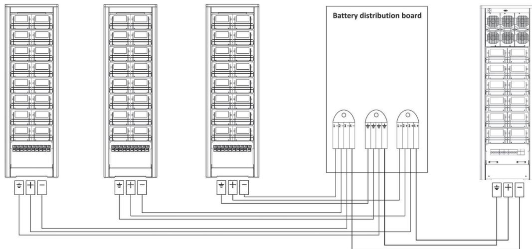
The external modular battery cabinets must be connected to the switchboard with the multipolar cables provided.
